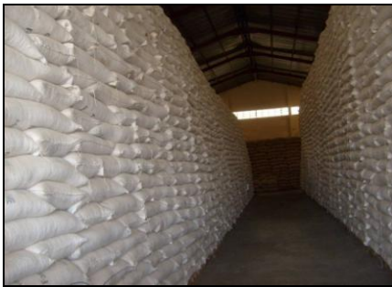
A stack of polypropylene bags; note the space between the stacks, the use of pallets and the use of the three unit stacking method.
