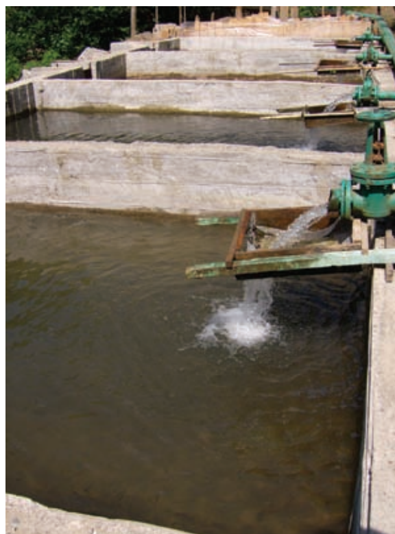
Fig. 2. Typical concrete single-pass trout rearing tanks in the Lesser Caucasus mountain region of Southern Georgia. Photo by Michael A. Rice.
